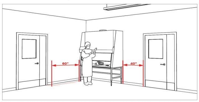
Placing BSCs near doorways is not recommended. If this arrangement is absolutely necessary maintain a distance of 40" to adjacent doorways and 60" to doorways behind the BSC.
